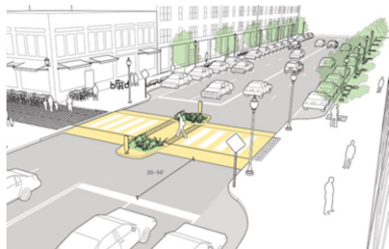
IMAGE: Example of mid-block crosswalk (National Association of City Transportation Officials)
