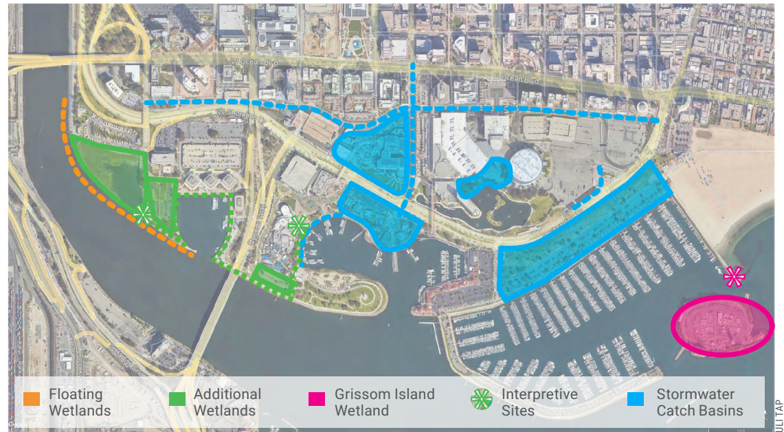
Floating wetlands and enhanced stormwater catch basins could enhance the waterfront's resilience.
