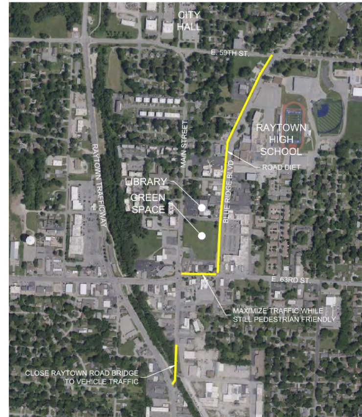
Roadway improvements to segments highlighted in yellow could include a road diet near the high school and closing the wood bridge to traffic near the community corridor.
