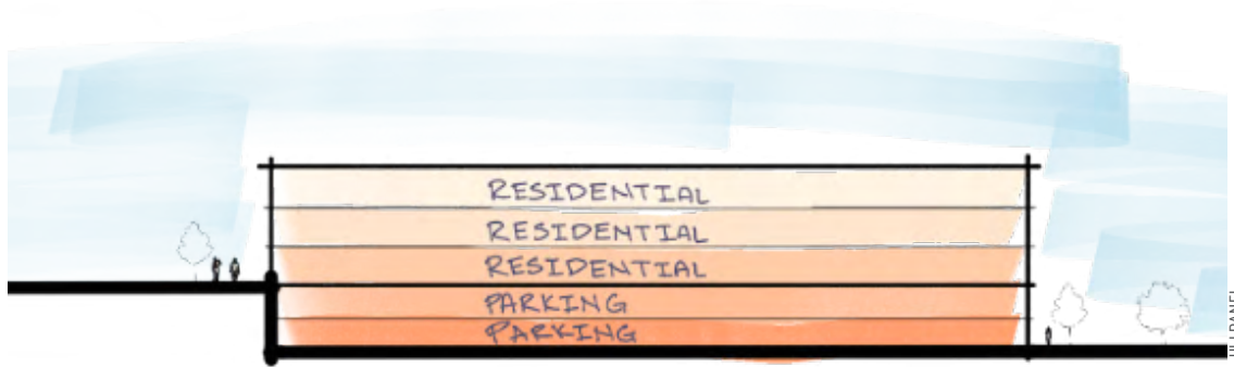
Using the topography on the western side of the study site, a building could tuck parking into the hillside and position all residential spaces above grade.
