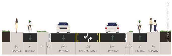
A cross-section of the roadway in the complete streets plan shows how the current roadway could be reconfigured to make space for all modalities passing safely along the corridor together.
