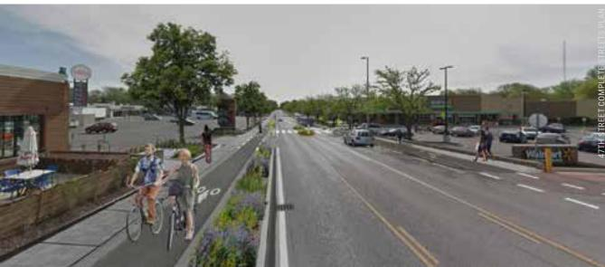
TOP: The 2018 complete streets plan shows how restriping the traffic lanes to reduce the number of auto lanes to create space for bicyclists can be achieved in the short term. BOTTOM: A possible approach to creating a complete street on Rainbow Boulevard could include raised infrastructure to separate bicyclists and pedestrians from the roadway.
