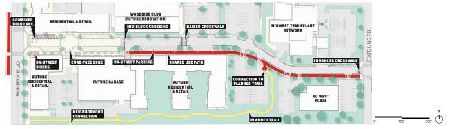
A proposal for West 47th Place demonstrates how the roadway can both serve the surrounding developments' auto needs as well as create space for on-street parking, multiple crosswalks, and bike/ped connections to shared-use paths and trails.
