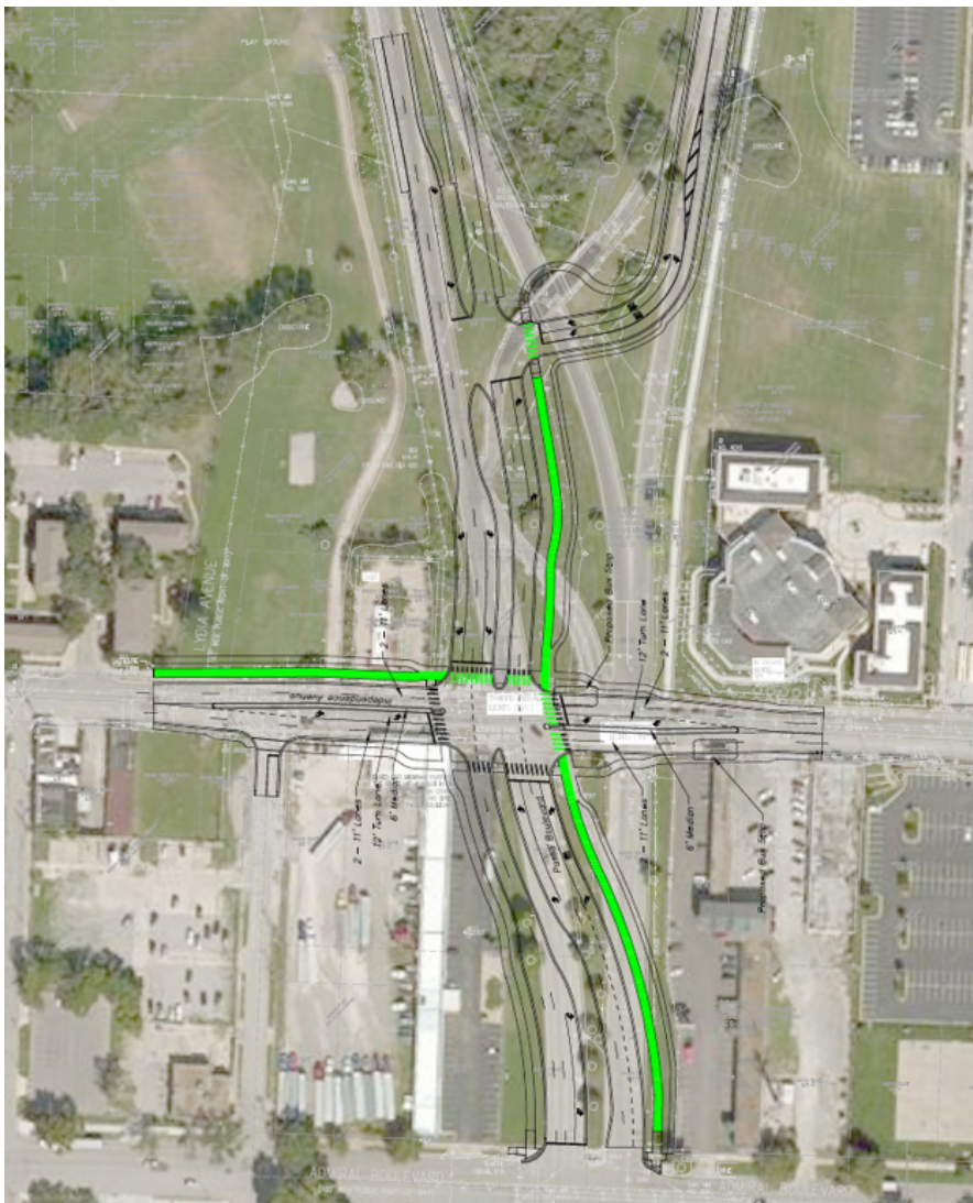
The redesign of the Independence Ave. and The Paseo intersection, due to start in late 2020 or early 2021, will straighten a dangerous and confusing roadway. Source: TAP Panel.
