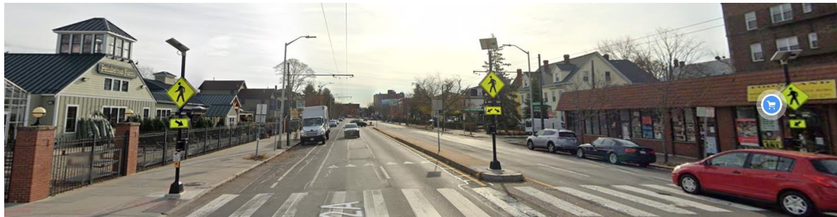
Rectangular Rapid Flashing Beacon, Massachusetts Avenue, Cambridge, MA
