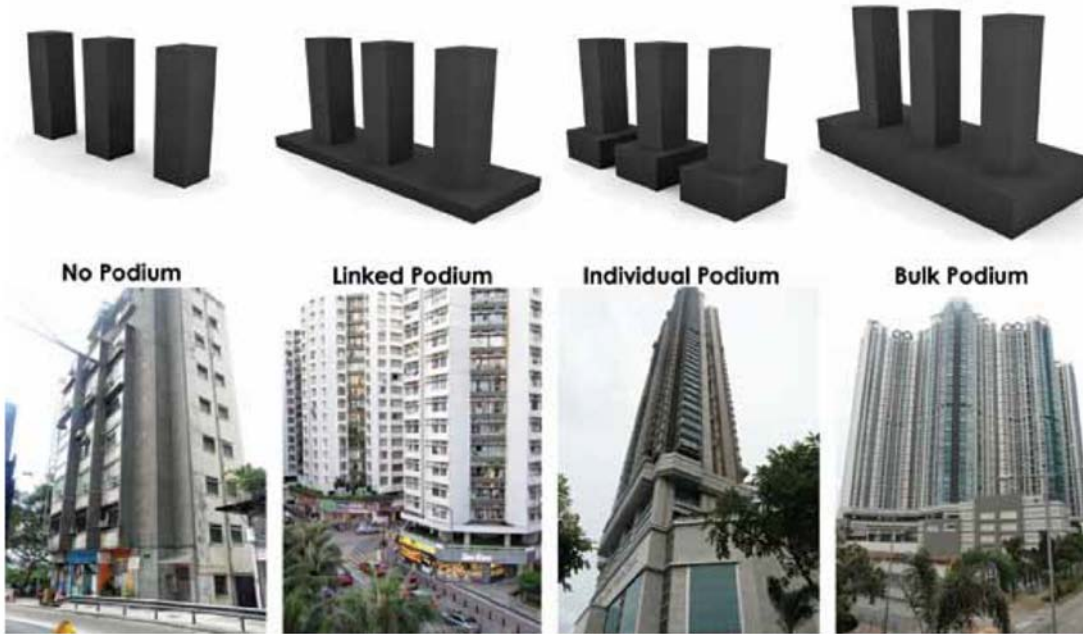
One of the dilemmas facing the city is the use of large, uninterrupted bulk podiums. Safeguards against such designs can be incorporated into the local area plan.
