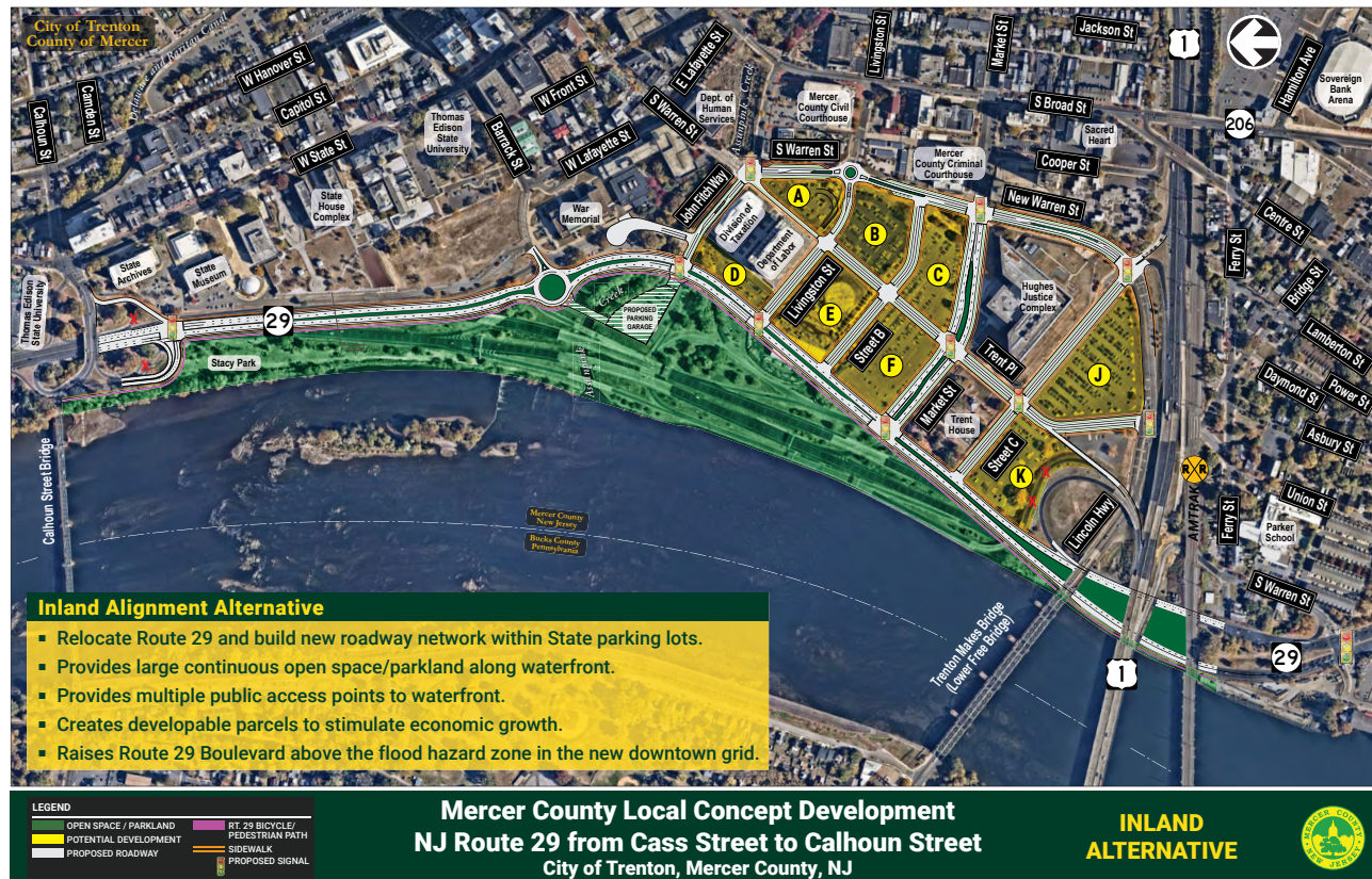
This design concept reroutes NJ29 inland, creating an expanded riverfront park and more connected street grid.
