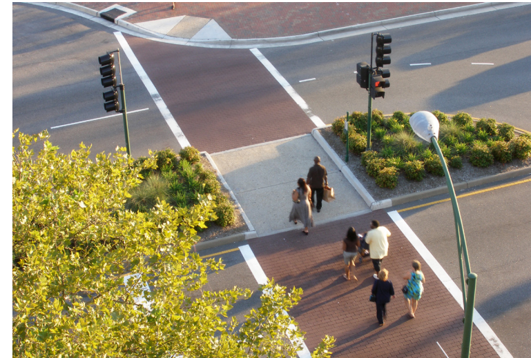
Pedestrian crosswalks can be colorful, textured, raised, and divided, all of which call attention to the space, encouraging drivers to slow down and helping protect the pedestrians moving through the area.
