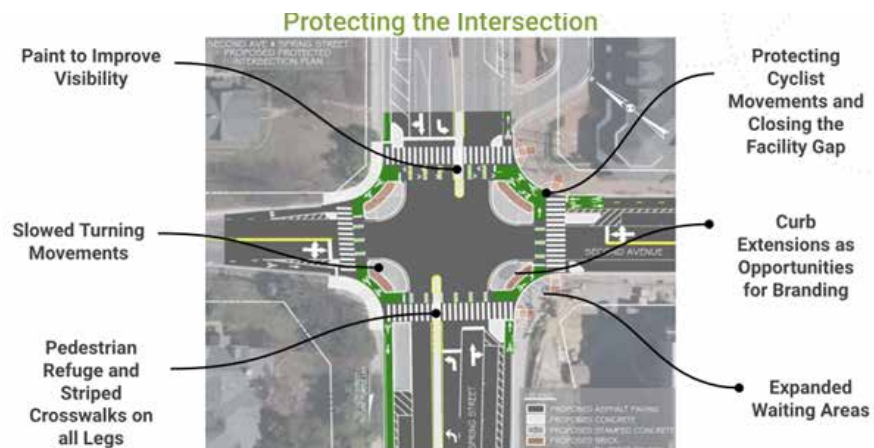
An example of a Dutch junction, a safer intersection that the Panel proposes for Key Highway
