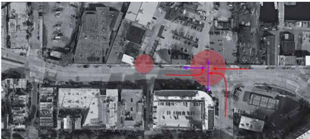
Existing Intersection and Entrance: The small red dot is the current egress. The larger red dot is where the crossing conflict occurs with turning vehicles.
