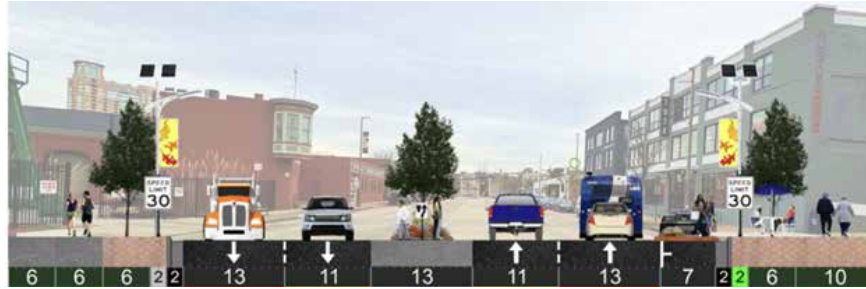
Updated street section of Key Highway, proposed by the Panel
