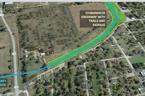
Green stormwater infrastructure along Caney Creek can simultaneously address stormwater runoff and provide the community with recreation opportunities. Source: Google Earth with Panel notations.
