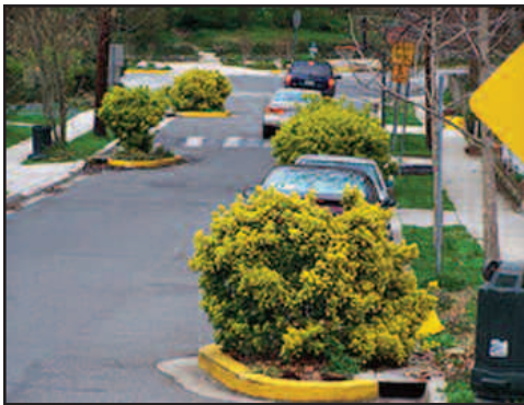
(Figures 12a & 12b) Bulb-outs can create a perceived narrowing of the road, which can help reduce vehicular speed.
