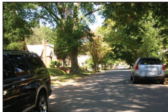
(Figure 8) Tertiary streets are the least traveled of all types and should have on-street parking.
