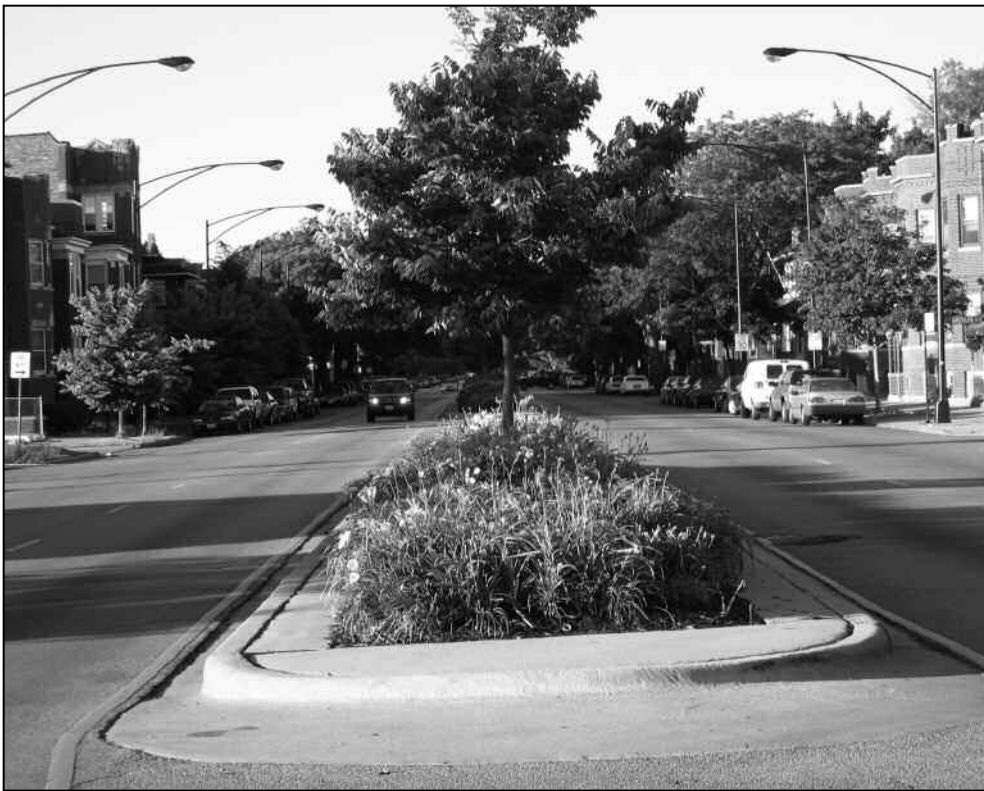
Figures 8 Decorative medians help break up wide streets and make them more pedestrian friendly.
