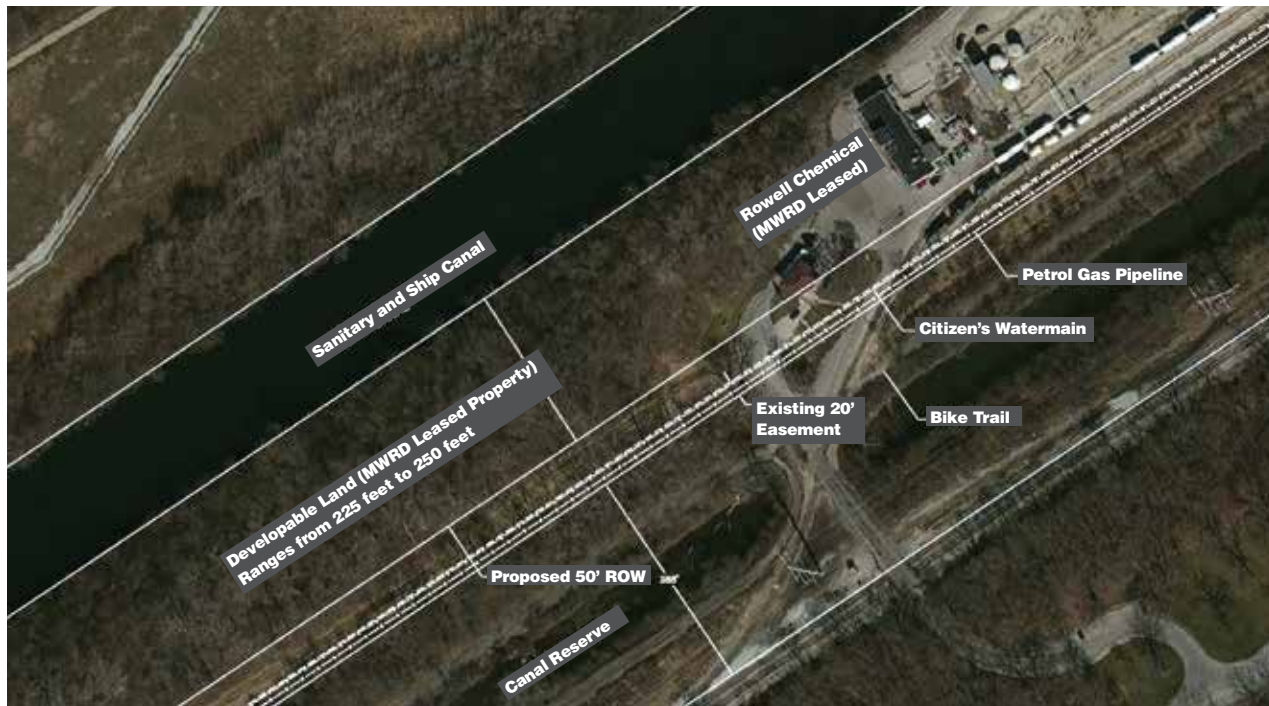
Figure 4: Easements and Right-Of-Way within the study corridor
